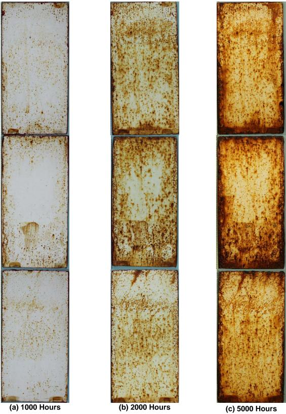
Figure 1. Images of the Three SUPER THERM Coupons After (a) 1000, (b) 2000, and (c) 5000 Hours of Exposure
