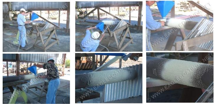
A temperature reduction from 370°C on the bare pipe to 90°C after the second primer coat @ 50 mils DFT. (Video)
