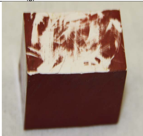
(h) Removing a layer of coating
