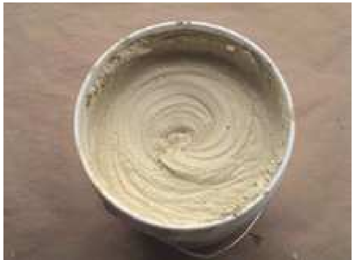
After Proper Mixing / Ready to Apply
