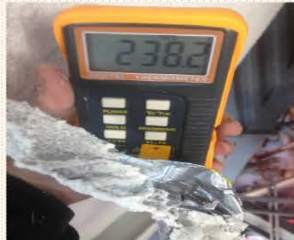
Final coat specified thickness 275 – 300 mils DFT Both top and bottom thermocouple readings the same.
